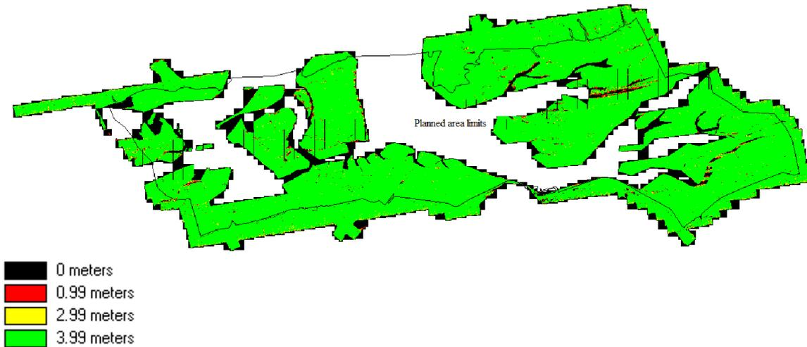
**Figure 8.3 and 8.4** are giving the same overview, only including big water areas this time. Average pointdensity including big water areas is 6.5 pts/m<sup>2</sup> and within the area 80.85% of the cells have a pointdensity of 4 pst/m<sup>2</sup> or higher.
