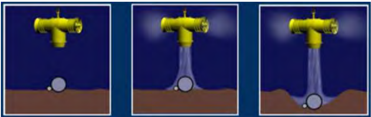
Figure 43 Mass flow excavation
