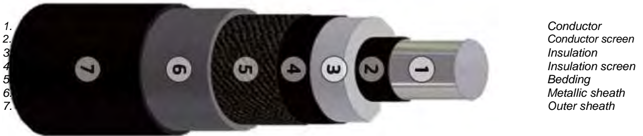
Figure 6 Typical HVAC 220 kV land export cable
