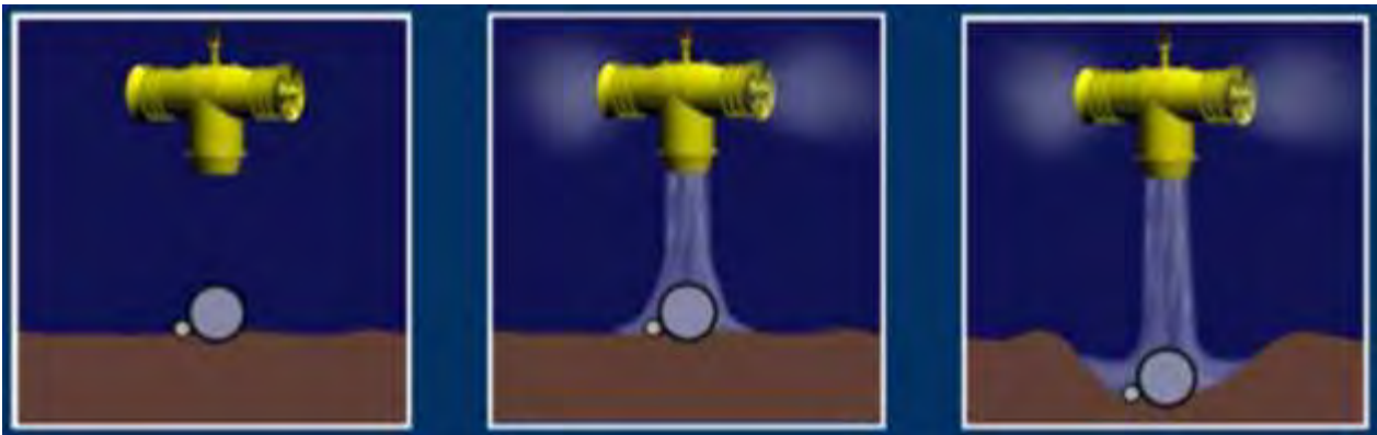
Figure 43 Mass flow excavation
