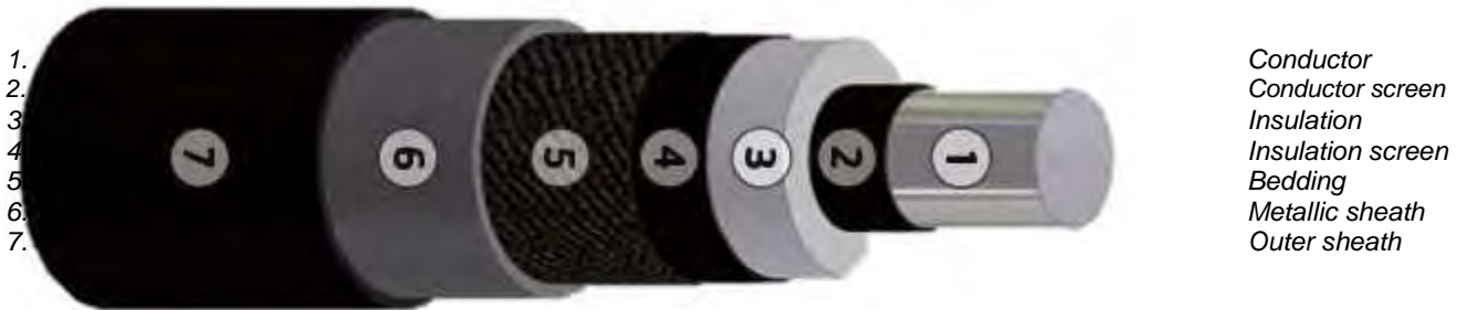
Figure 6 Typical HVAC 220 kV land export cable
