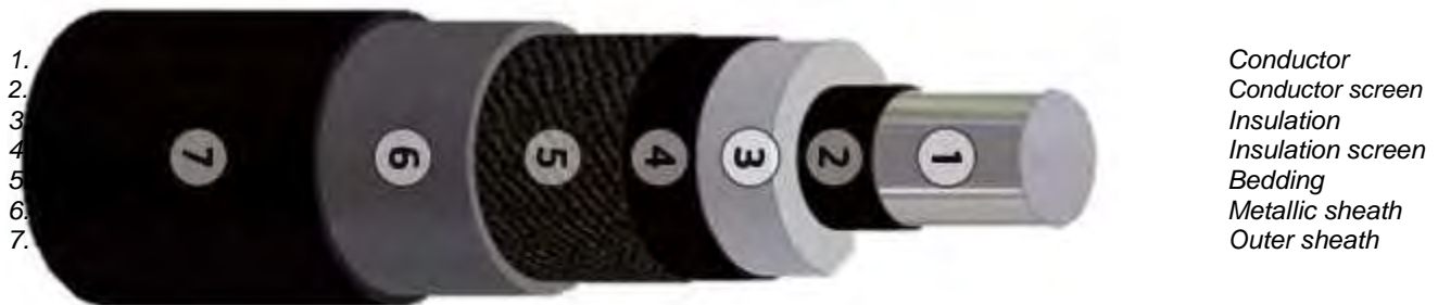
Figure 6 Typical HVAC 220 kV land export cable
