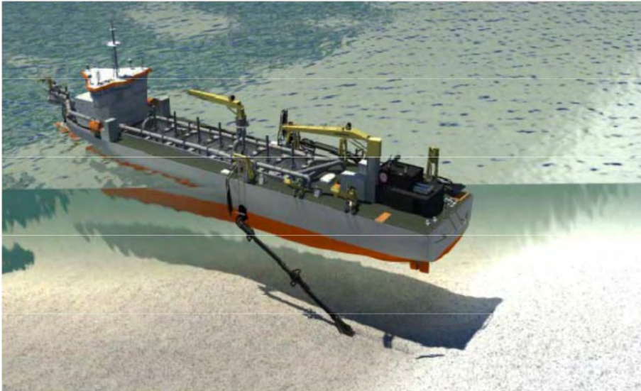
Figure 52 Trailing Suction Hopper Dredger
