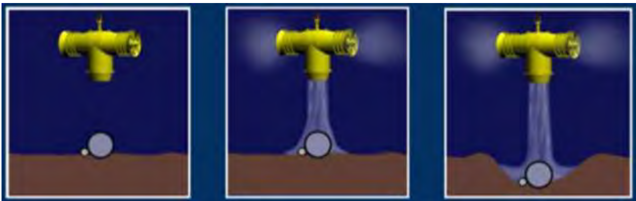
Figure 43 Mass flow excavation
