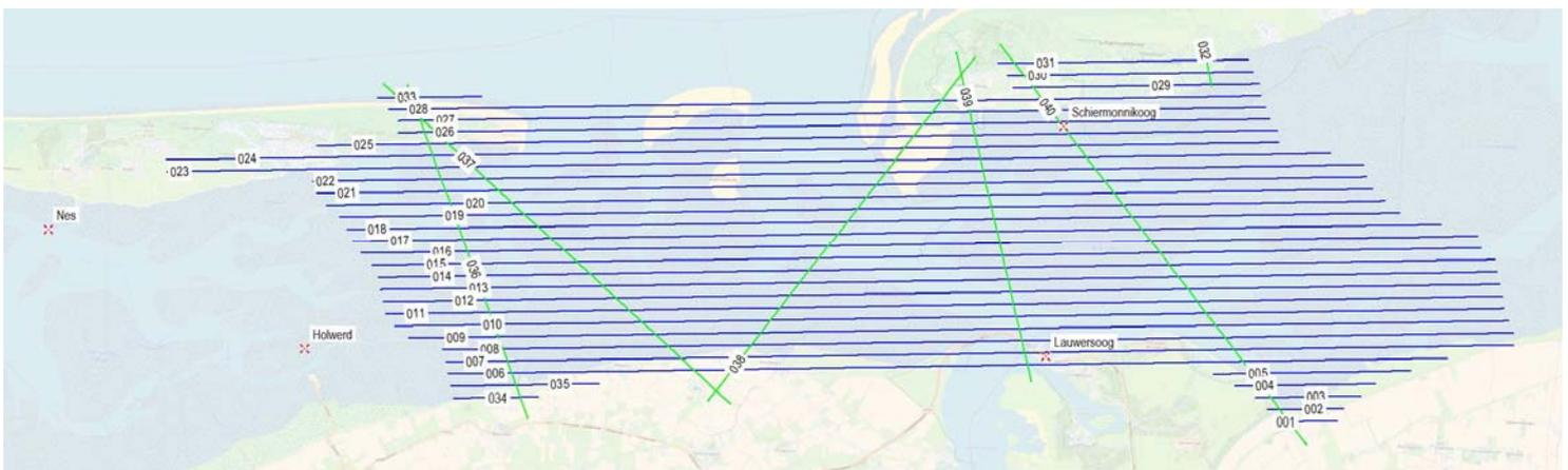
Figure 4: Flightplan and waterlevel stations
