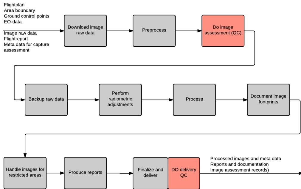
Figure 13: Image processing from raw data download to data delivery
