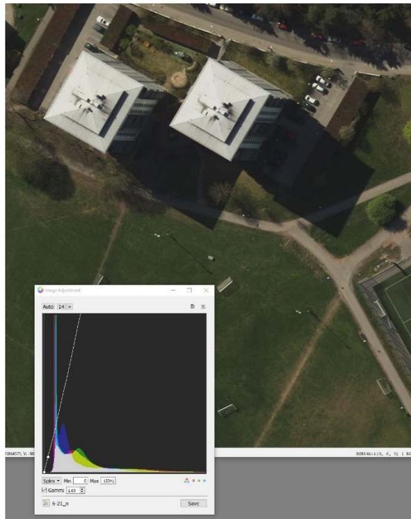
Figure 16: Screenshot of adjusting radiometric profile in HxMap
