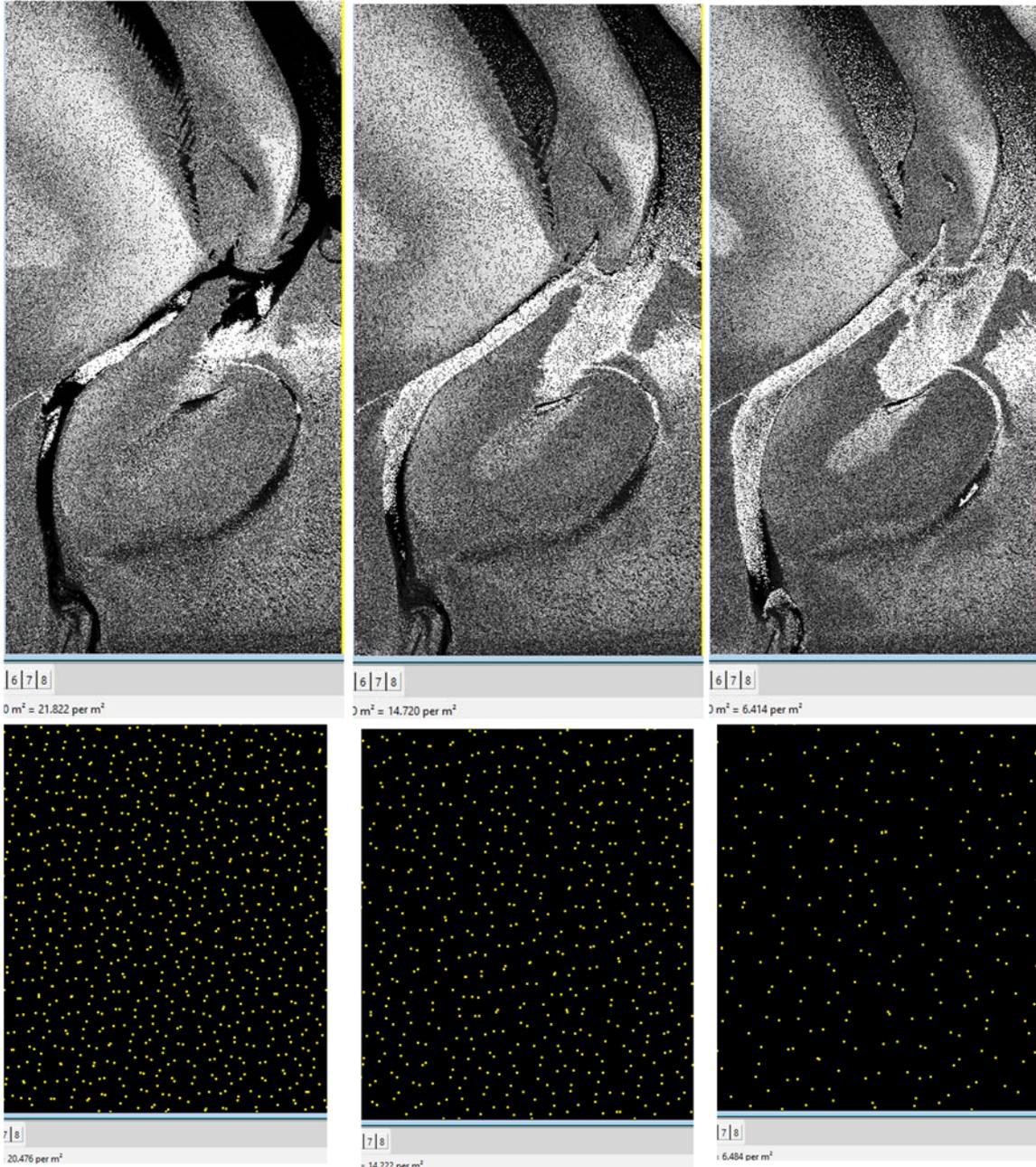
Figure 12: Images on the top shows how the terrain attributes are kept with increasing flight height and lower density. The lower images show an even distribution of laser points with decreasing density due to higher flight height.
