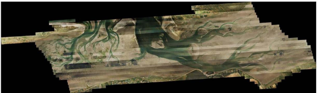
*Figure 14: Mosaic of project after corrections including atmospheric correction and Multiframe color balancing*
