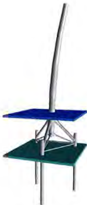
Figure 5-5 Integrated structure in 1. bending mode
