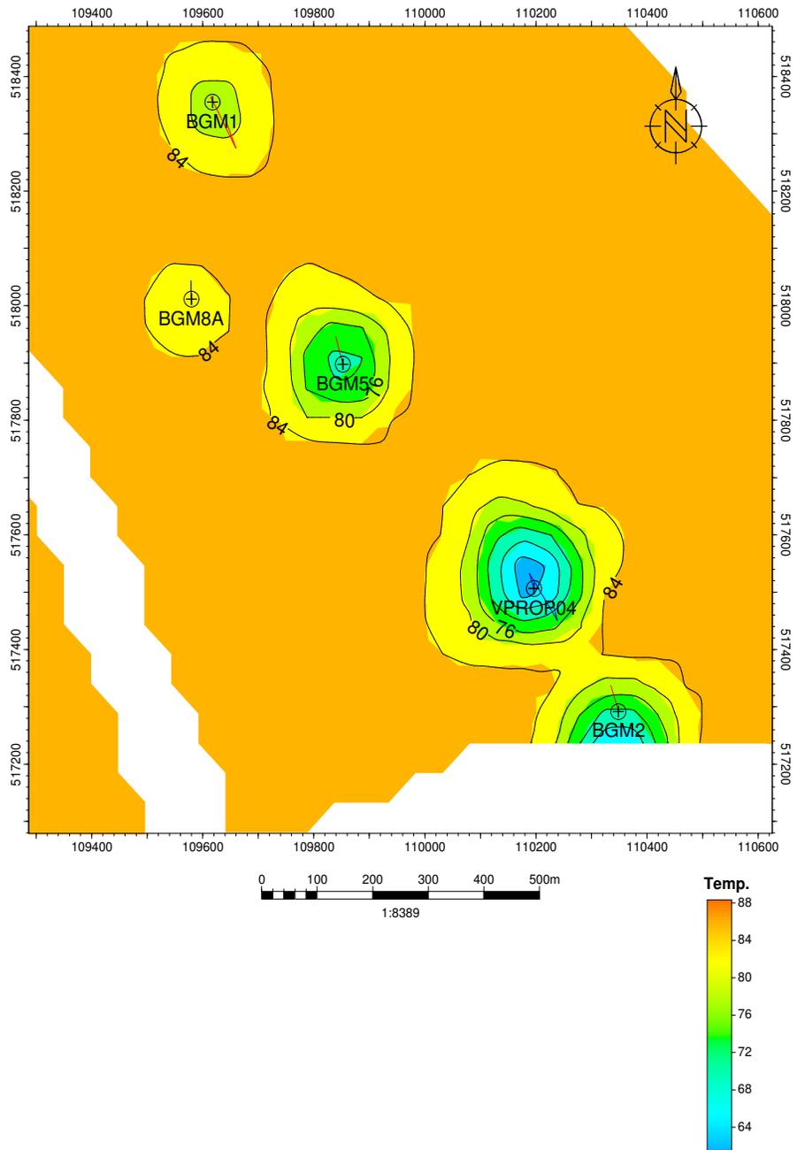
Figure 5.3: Temperature distribution at 24<sup>th</sup> of October for layer 13. Although this is just after the first cushion gas injection period, the lowest temperatures are reached at this date as 1) injection gas temperature is lowest at 20-30°C, as compared to 60-66°C in later phases, and 2) injection rates per well are high as only 6 wells are injecting, while in later phases up to 17 wells are injecting.
