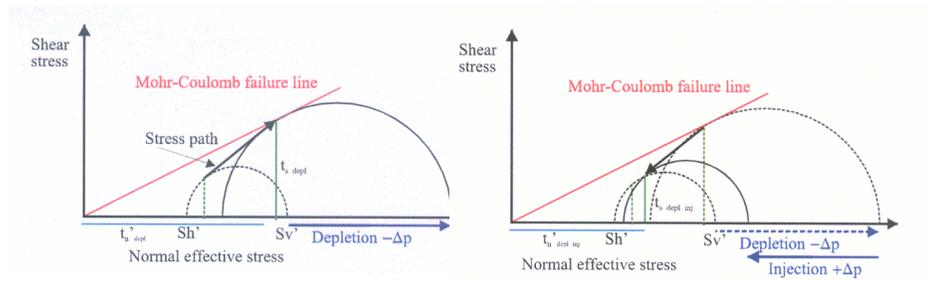
Figure 6.3: Left: Critical development of the stress path for depletion. Right: Non-critical development of the stress path for injection in a depleted reservoir.
