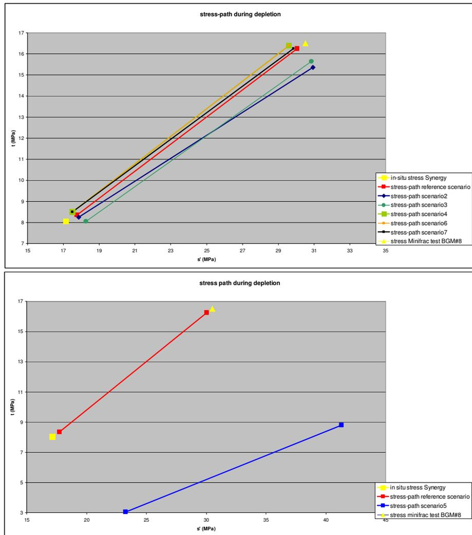
Figure 6.14: Stress-paths during depletion. Stresses at the start and end of depletion are plotted. In the top figure the stress paths for the reference scenario and scenario's 2, 3, 4, 6 and 7 are plotted (no creep). The bottom figure gives the stress path for scenario 5 (creep Zechstein).
