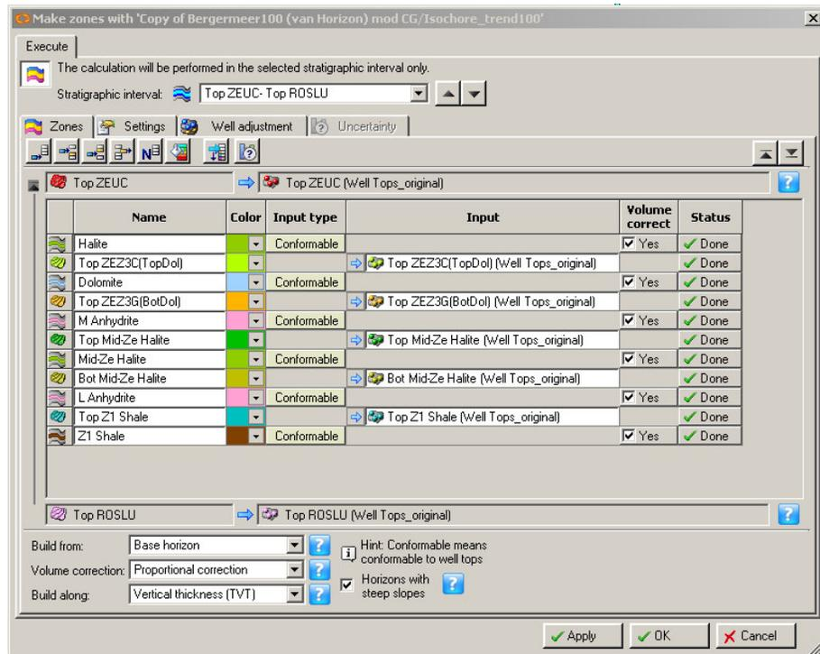
Figure 3.5: Parameters used in the zone building process of the separate Zechstein Petrel model.
