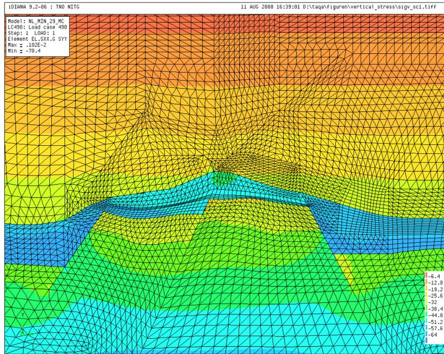
Figure 6.9: In-situ vertical effective stresses [MPa] in and around the reservoir – *reference* scenario 1.
