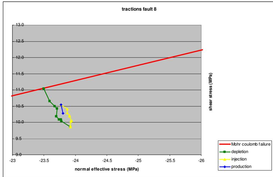
Figure 6.24: Stress path on overburden fault 8. Reference scenario 1.
