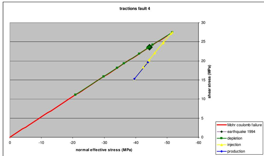
Figure 6.16: Stress path on fault4, in fault element 160 halfway the overlap of reservoir rocks. Reference scenario 1.
