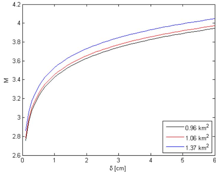
Figure 2.3: The relation between the magnitude of a seismic event and the slip displacement for the southwestern (0.96 km<sup>2</sup>), internal (1.06 km<sup>2</sup>) and northeastern (1.37 km<sup>2</sup>) fault of the Bergermeer field.
