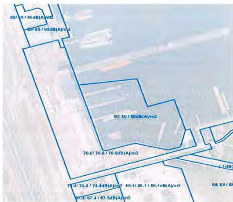
Figuur 3.1: Geluidsbudget Botlek Tank Terminal (in d(B)A/m 2 ) [Bron: DCMR]
