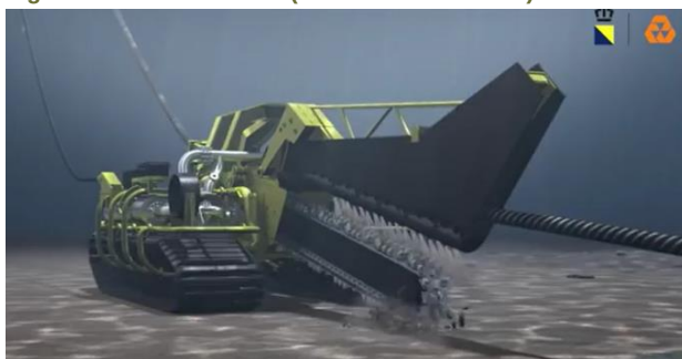
Figuur 2.12 Chain cutter (trench former VBMS)
