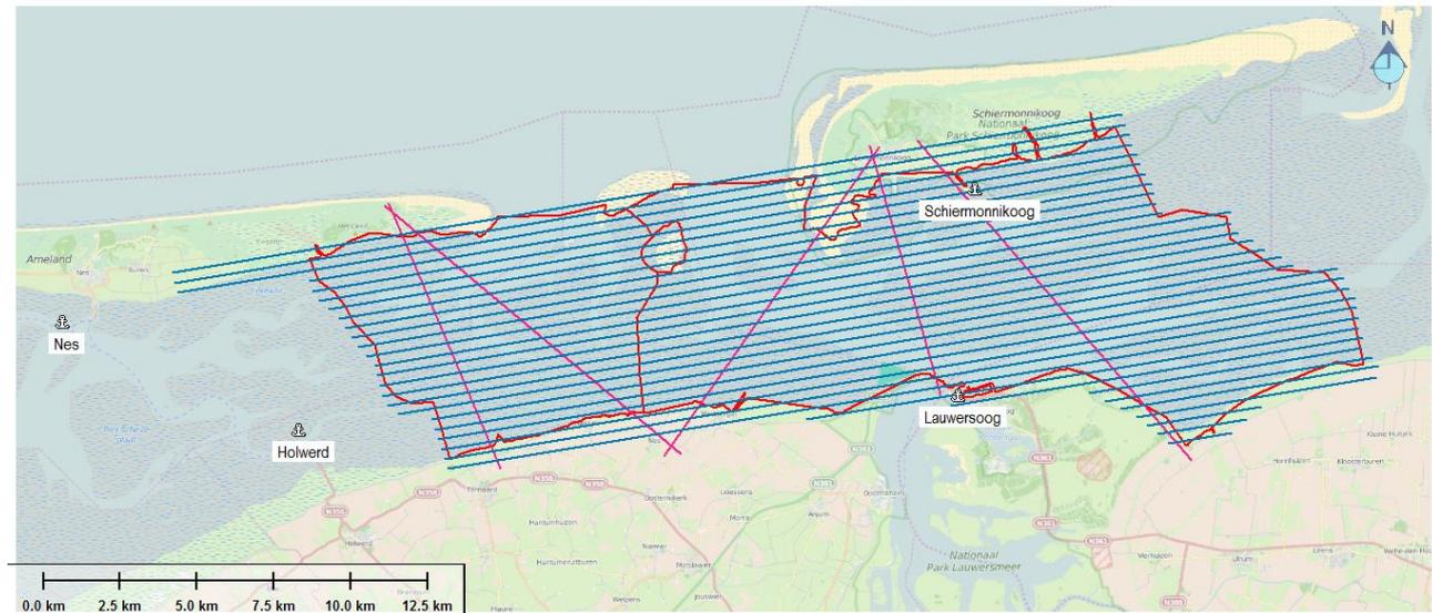
**Figure 1: Project area, flightlines, and tidal stations**
