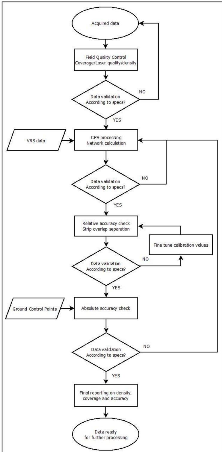
Figure 5: Processing flowchart
