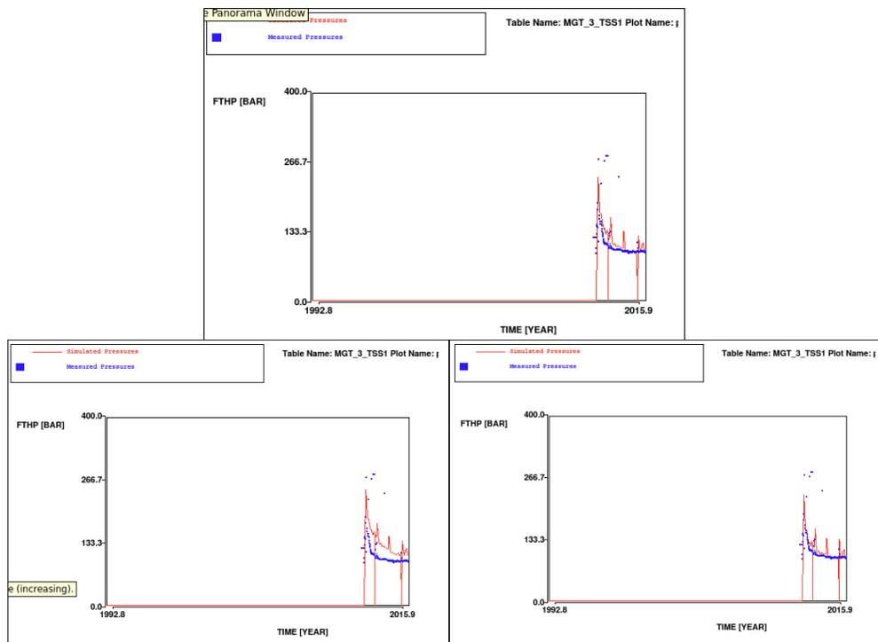
Figure 62 Simulated (red line) and measured (blue squares) flowing tubing head pressures in MGT-2. Top: Bes case. Left: low case. Right: high case.
