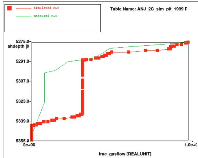
Figure 41 Simulated (red line + squares) and measured (green line) PLT in ANJ-2C in 1999 with original perforations from 1994 closed and new perforations from 1997 added. Base case realisation.
