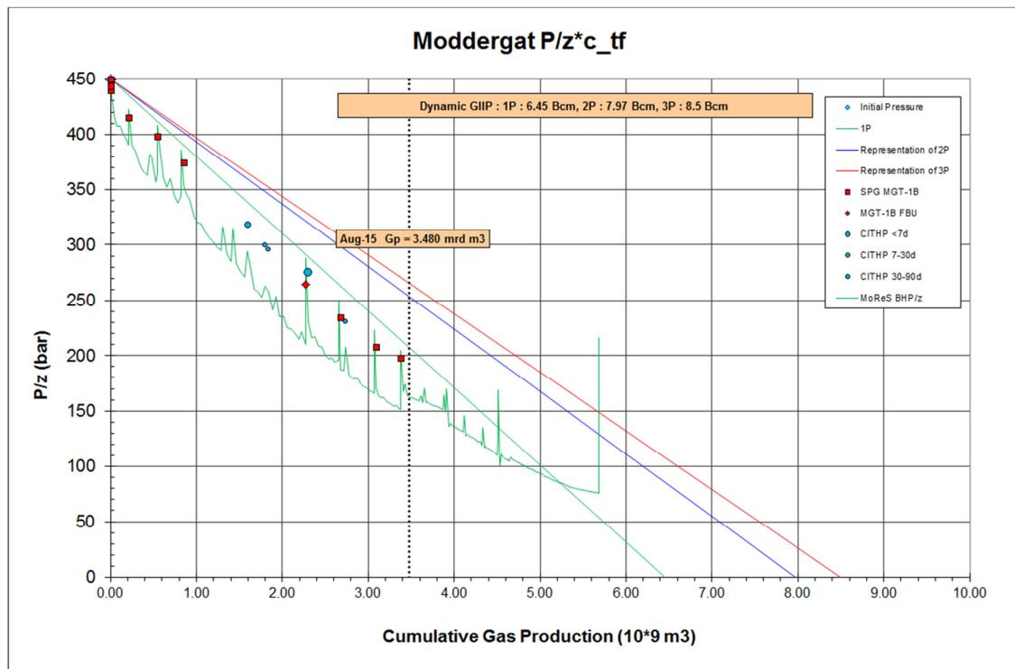
Figure 49 P/z plot for MGT-1B.
