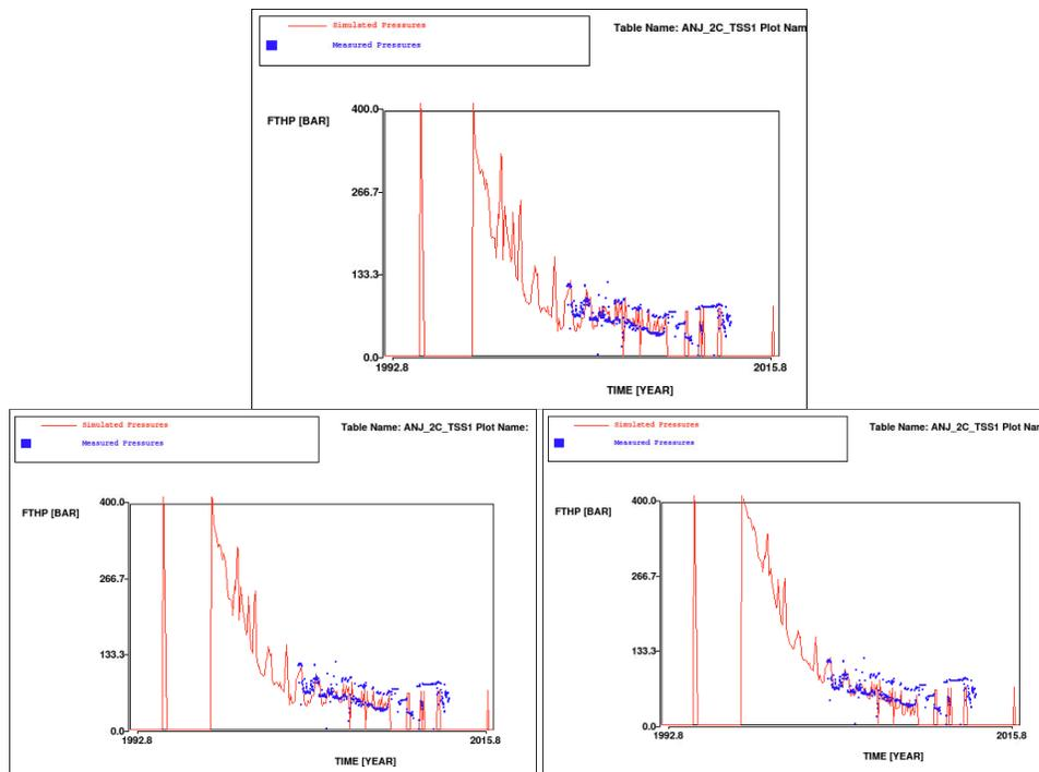
Figure 42 Simulated (red line) and measured (blue squares) flowing tubing head pressures in ANJ-2C. Top: base case. Left: low case. Right: high case.
