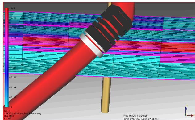
Figure 45 Cross section of the water saturation change around ANJ-2C with in red the water entering via high permeable streaks and cross flowing at the top (blue is no change in saturation).
