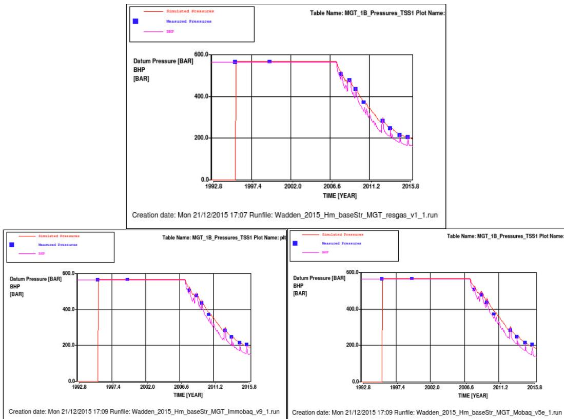
Figure 51 Simulated reservoir pressure (red line), simulated BHP (violet line) and measured (blue squares) downhole pressure data in MGT-1B. Top: base case. Left: low case. Right: high case.
