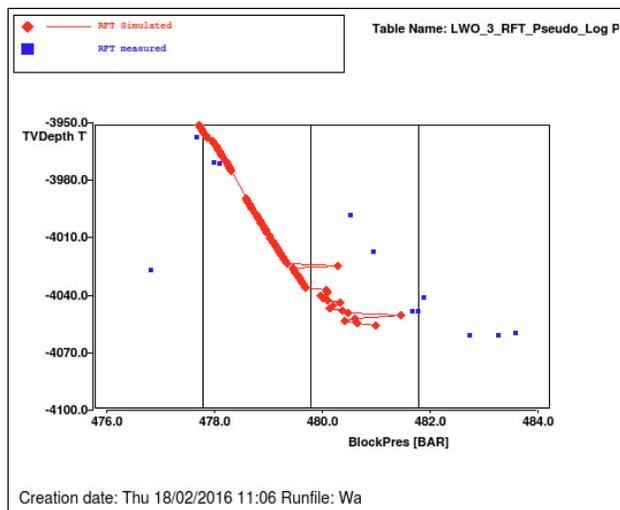
Figure 32 Simulated (red line and squares) and measured RFT pressure data (blue squares) for LWO-3.
