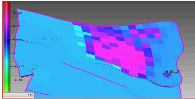
Figure 46 Water saturation change in unit 1, with in red the water encroaching from the west (blue is no change in saturation), and around the well the cross-flow.
