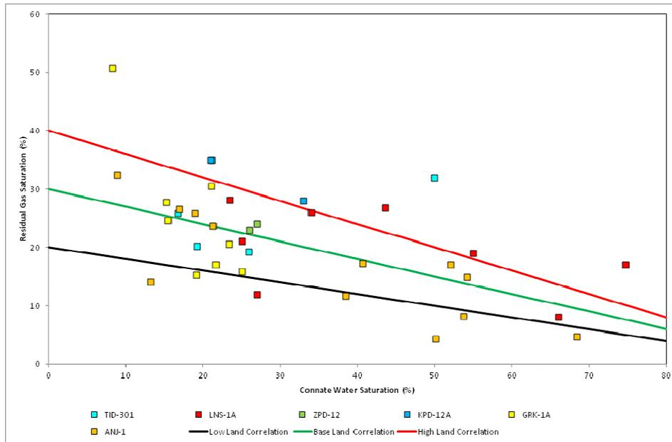
Figure 3 Residual gas saturation as a function of the connate water saturation
