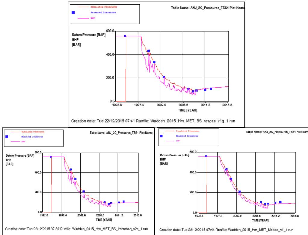
Figure 43 Simulated reservoir pressure (red line) and measured (blue squares) downhole pressure data in ANJ-2C. Top: base case. Left: low case. Right: high case.
