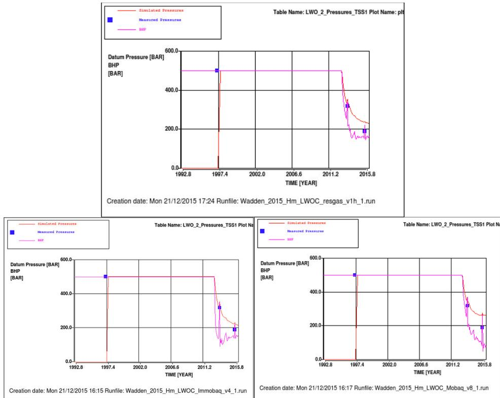
Figure 21 Simulated pressure (red line ), simulated BHP (violet line) and measured (blue squares) downhole pressure data in LWO-2. Top: base case. Left: low case. Right: high case.
