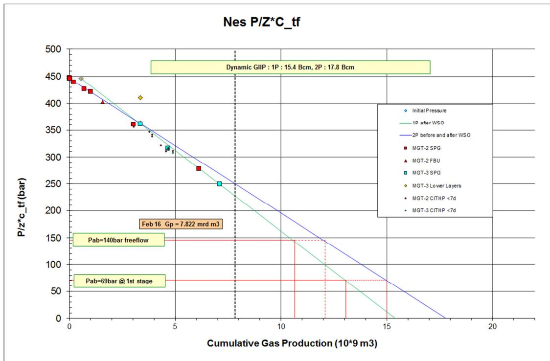
Figure 56  $P/z$  plot for MGT-2 and MGT-3. Due to the high initial pressures,  $P/z$  has been corrected for rock compressibility ( $c_f$ ).
