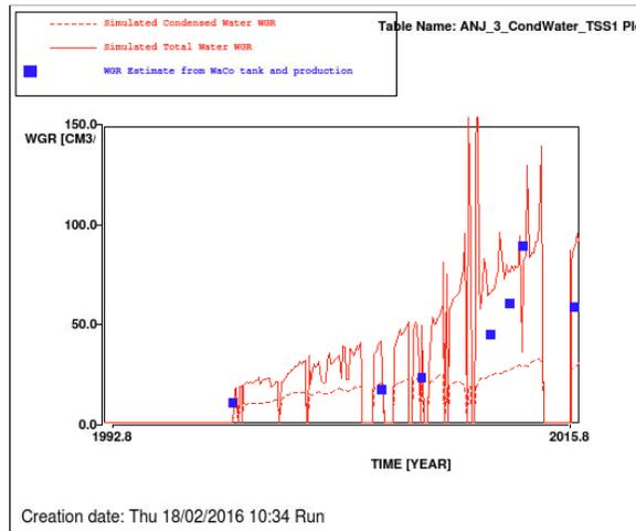
Figure 18. Simulated total WGR (red solid line), simulated condensed WGR (red dashed line) and estimated WGR from production and WaCo tank observations (blue squares) for ANJ-3. Base case realisation.
