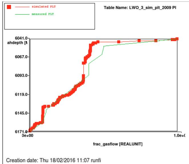
Figure 33 Simulated (red line + squares) and measured (green line) PLT in LWO-3. Base case realisation.
