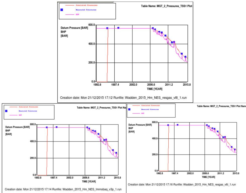
Figure 59 Simulated reservoir pressure (red line), BHP (violet line) and measured (blue squares) downhole pressure data in MGT-2. Top: Base case. Left: low case. Right: high case.
