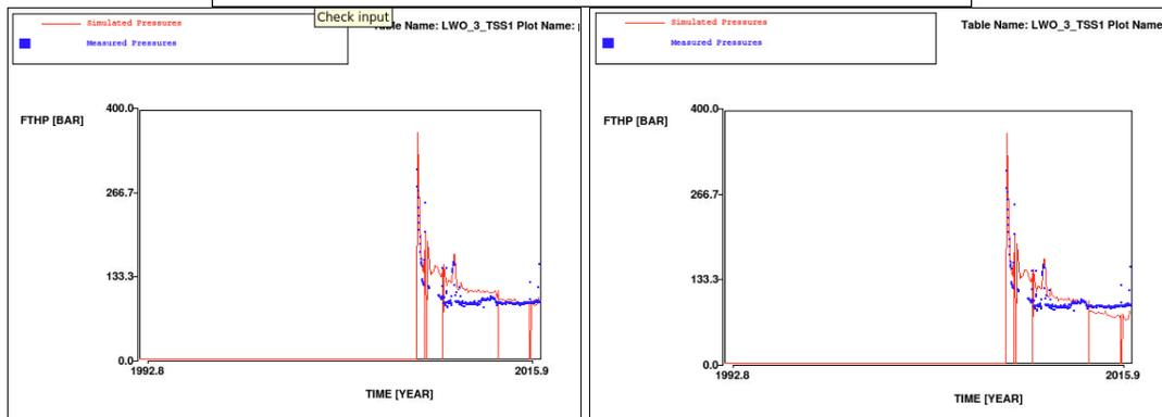
Figure 36 Simulated (red line) and measured (blue squares) flowing tubing head pressures in LWO-3. Top: base case. Left: low case. Right: high case.
