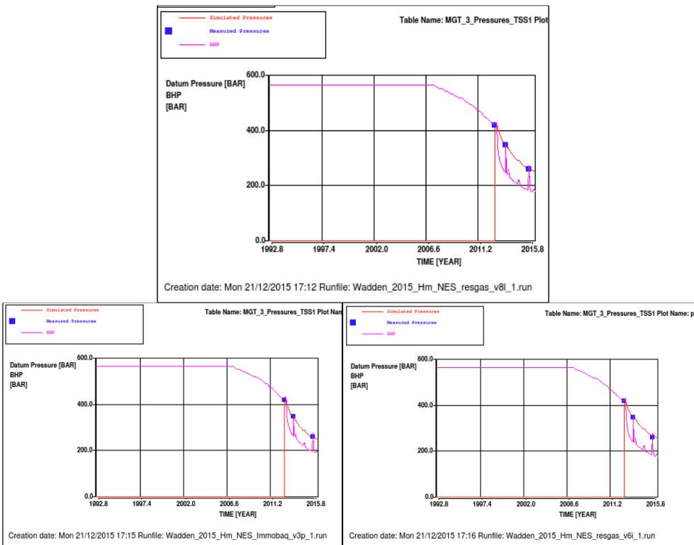
Figure 60 Simulated reservoir pressure (red line), BHP (violet line) and measured (blue squares) downhole pressure data in MGT-3. Top: Base case. Left: low case. Right: high case.
