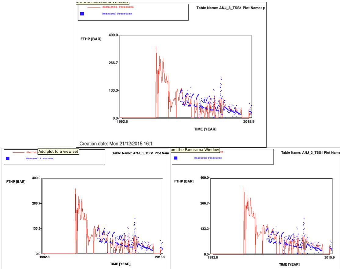
Figure 16 Simulated (red line) and measured (blue squares) flowing tubing head pressures in ANJ-3. Top: Base case. Left: Low case. Right: High case.
