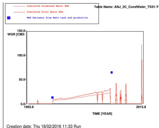
Figure 47 Simulated total WGR (red solid line), simulated condensed WGR (red dashed line) and estimated WGR from production and WaCo tank observations (blue squares) for ANJ-2C
