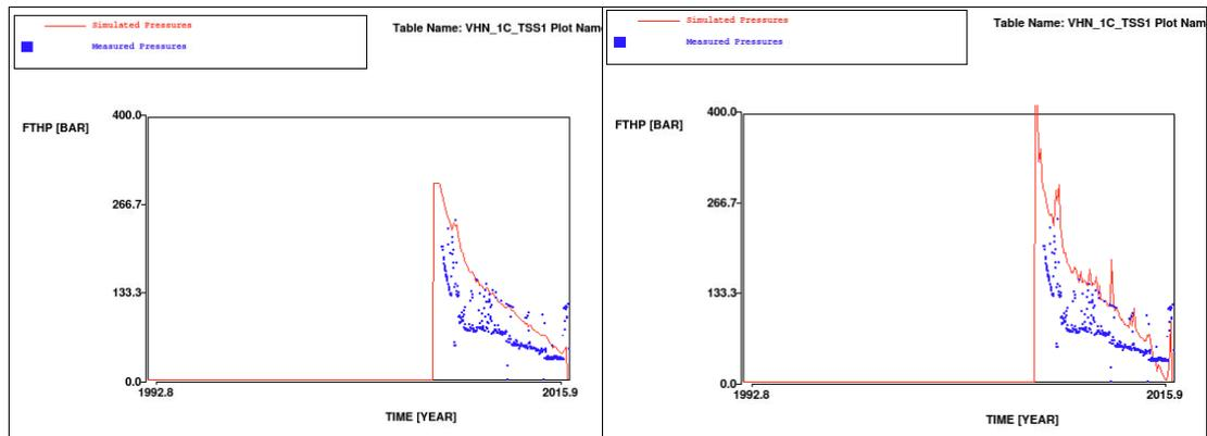
Figure 67 Simulated (red line) and measured (blue squares) flowing tubing head pressures in VHN-1C. Left: low/base case. Right: high case.
