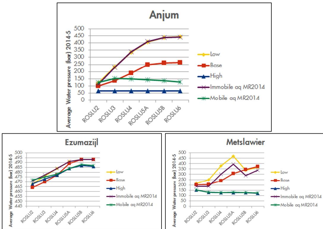
Figure 72 Water pressures in 2015, per zone for fields Anjum, Ezumazijl and Metslawier.
