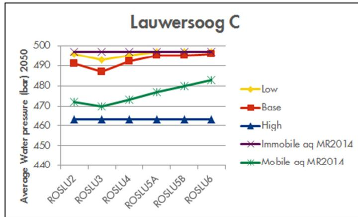
Figure 73 Water pressures in 2050, per zone for Lauwersoog C.
