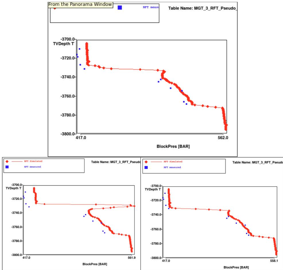
Figure 58 Simulated (red line and squares) and measured RFT pressure data (blue squares) for MGT-3. Top: base case. Left: low case. Right: high case.
