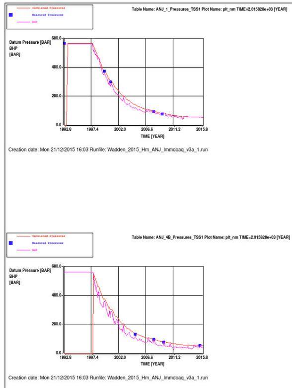
Figure 8 Simulated pressure (red line), simulated BHP (violet line) and measured down hole pressure (blue squares) for low case. Left: ANJ-1, Right: ANJ-4B.
