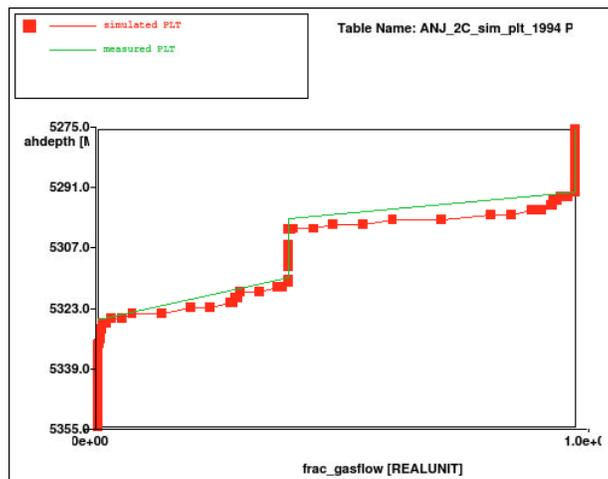
Figure 40 Simulated (red line + squares) and measured (green line) PLT in ANJ-2C with original perforations in 1994. Base case realisation.
