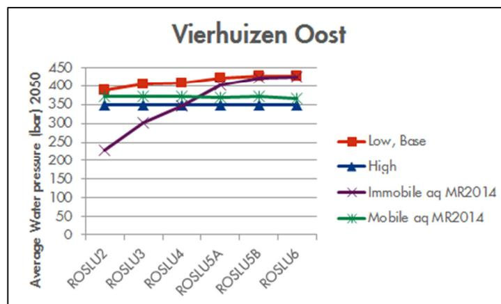
Figure 78 Water pressures in 2050, per zone for Vierhuizen.
