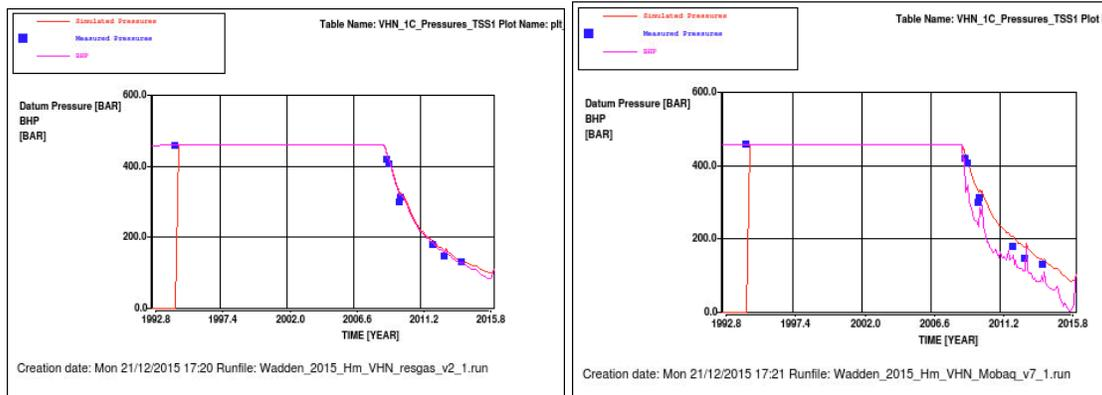
Figure 66 Simulated reservoir pressure (red line), BHP (violet line) and measured (blue squares) downhole pressure data in MGT-3. Left: low/base case. Right: high case.
