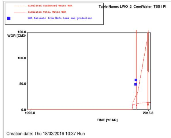
Figure 23 Simulated total WGR (red solid line), simulated condensed WGR (red dashed line) and estimated WGR from production and WaCo tank observations (blue squares) for LWO-2. Base case realisation.
