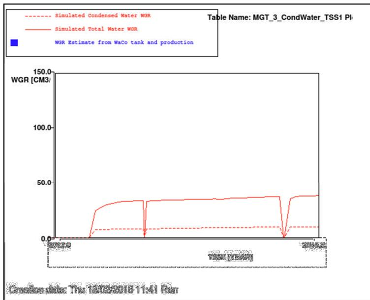
Figure 64 Simulated total WGR (red solid line), simulated condensed WGR (red dashed line) and estimated WGR from production and WaCo tank observations (blue squares) for MGT-3
