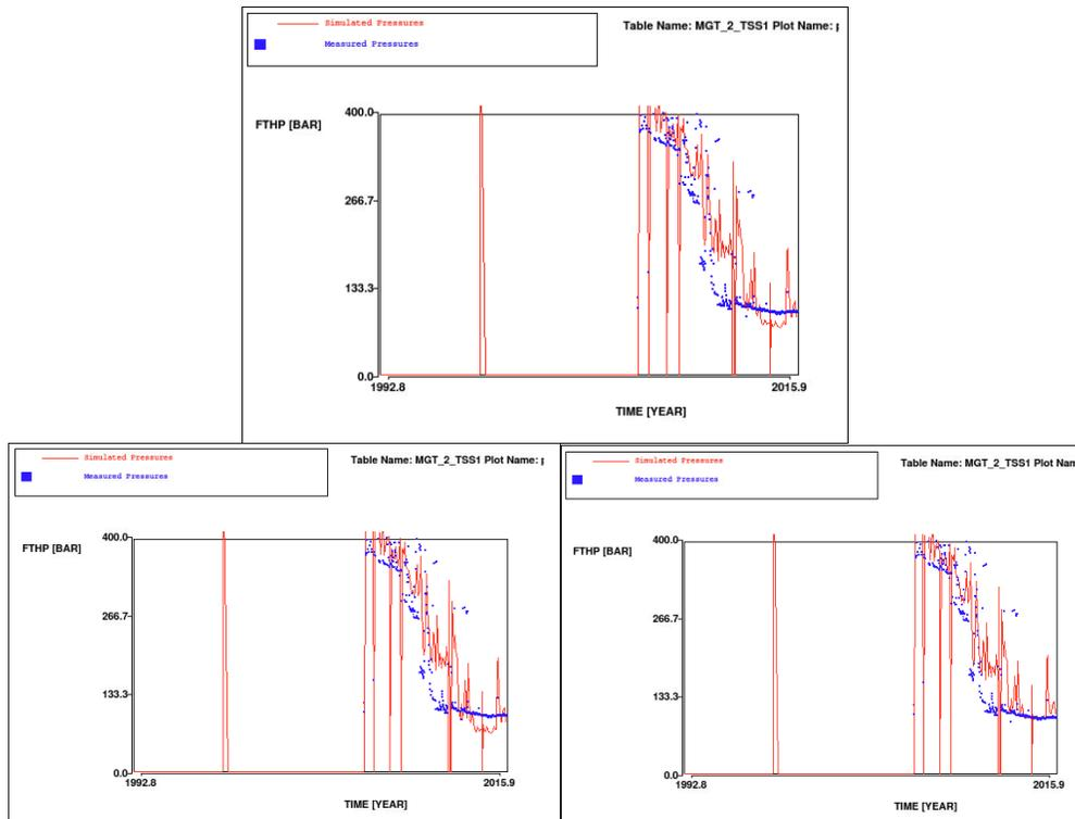
Figure 61 Simulated (red line) and measured (blue squares) flowing tubing head pressures in MGT-2. Top: Bes case. Left: low case. Right: high case.
