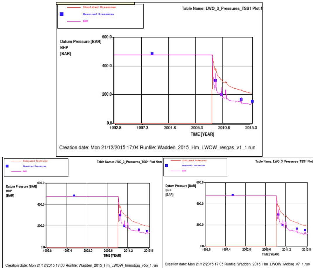
Figure 34 Simulated reservoir pressure (red line), flowing bottom hole pressure (violet line) and measured (blue squares) downhole pressure data in LWO-3. Top: Base case Left: low case. Right: high case.
