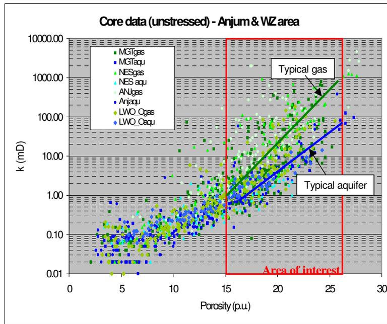
Figure 2 Core plug permeability data for gas and aquifer leg.
