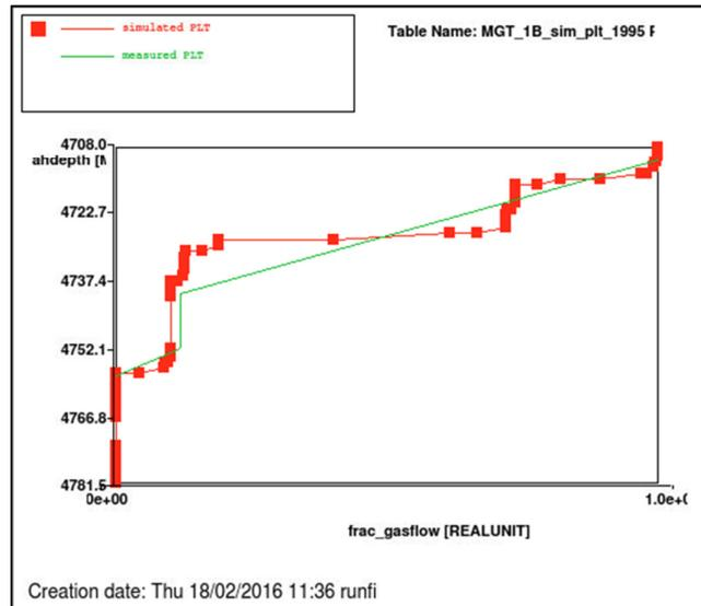
Figure 53 Simulated (red line + squares) and measured (green line) PLT in MGT-1B in 1995
