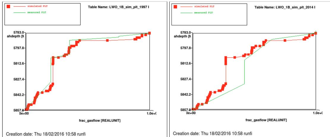
Figure 26 Simulated (red line + squares) and measured (green line) PLT in LWO-1B. Left: 1997, pre-production. Right: 2014. Base case realisation.
