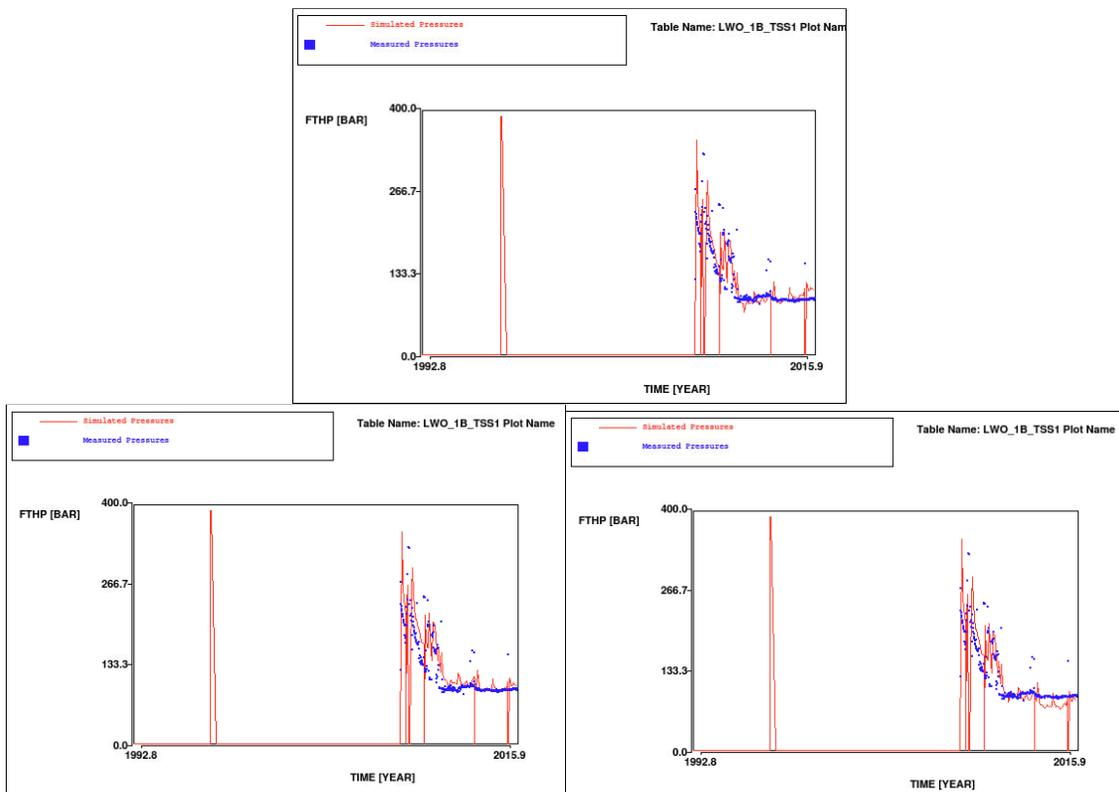
Figure 28 Simulated (red line) and measured (blue squares) flowing tubing head pressures in LWO-1B. Top: base case. Left: low case. Right: high case.
