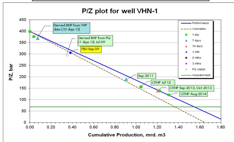
Figure 65 ARPR Top ROSLU map for Vierhuizen-East and P/z plot for VHN-1C.
