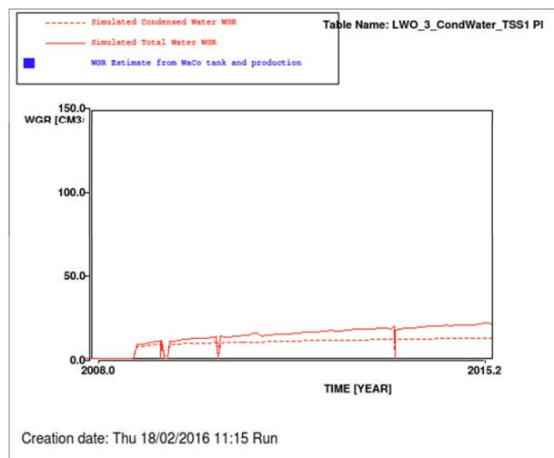
Figure 37 Simulated total WGR (red solid line), simulated condensed WGR (red dashed line) and estimated WGR from production and WaCo tank observations (blue squares) for LWO-3. Base case realisation.
