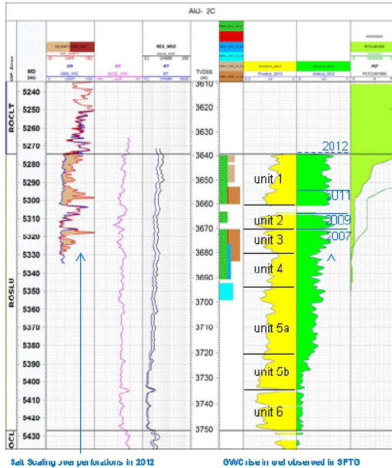
Figure 44 Log of ANJ-2C showing the salt scaling with the gamma ray log in the left panel and the liquid rise from SPTG in the right panel.
