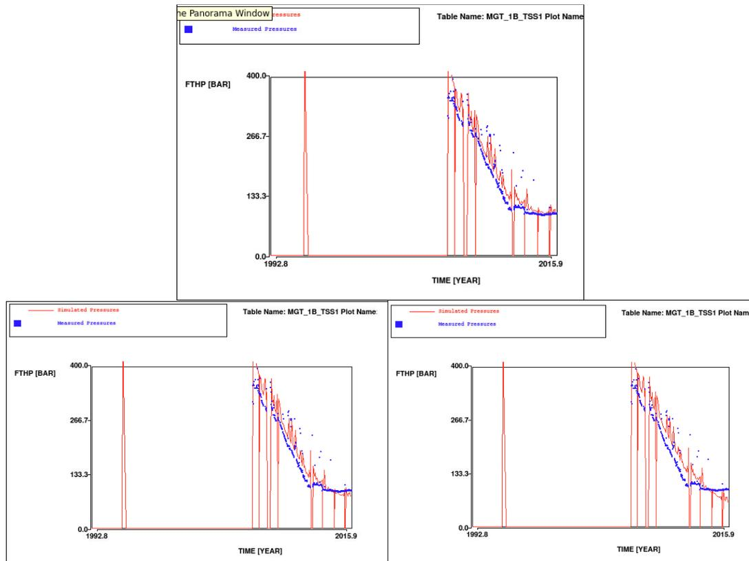
Figure 52 Simulated (red line) and measured (blue squares) flowing tubing head pressures in MGT-1B. Top: base case. Left: low case. Right: high case.
