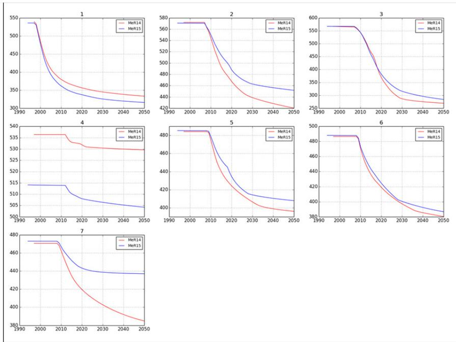
Figure 69 Average reservoir pressures per (set of) field(s), base case. Red: M&R2014, blue: M&R2015. 1 = Anjum, Ezumazijl, Metslawier, 2 = Moddergat, 3 = Nes, 4 = Lauwersoog Central (initial pressure modified due to gridding redefinition.), 5 = Lauwersoog East, 6 = Lauwersoog West, 7 = Vierhuizen East.
