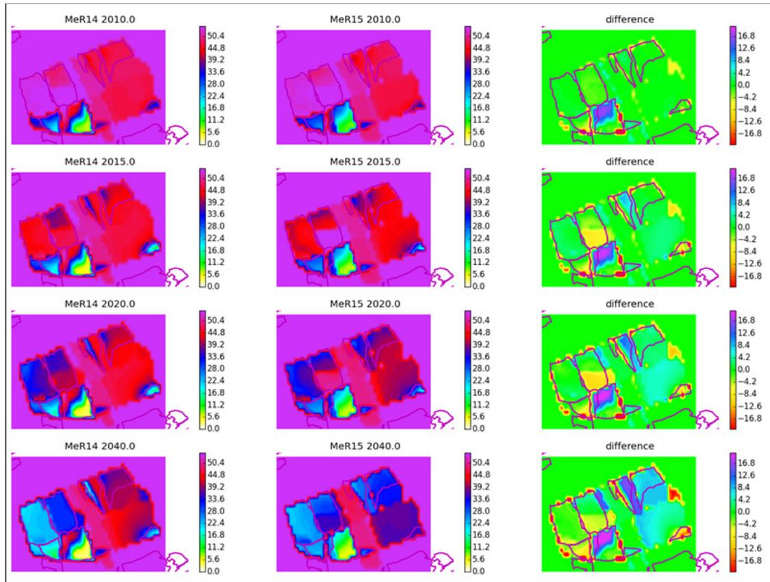
Figure 70 Modelled average reservoir pressure (MPa) Wadden area (high case). Left column: M&R2014. Middle column: M&R2015. Right column: difference plot. Top to bottom: 2010, 2015, 2020, 2050.
