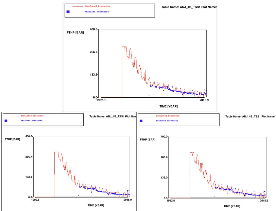
Figure 10 Simulated (red line) and measured (blue squares) FTHP data in ANJ-4B. Top: base case. Left: low case. Right: high case.
