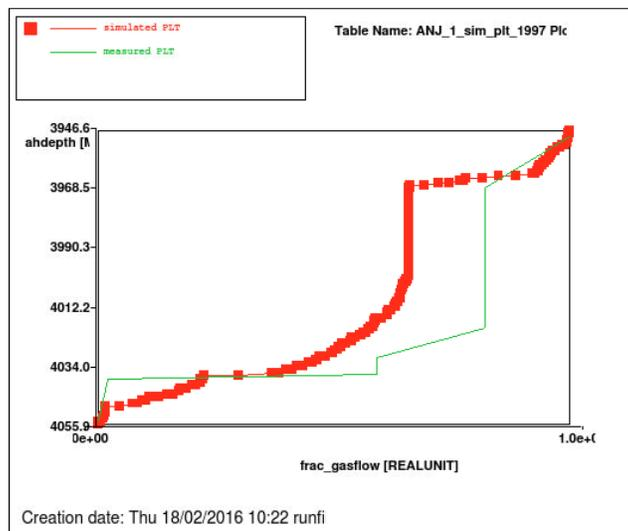
Figure 11 Simulated (red line + squares) and measured (green line) PLT in ANJ-1. Base case model.
