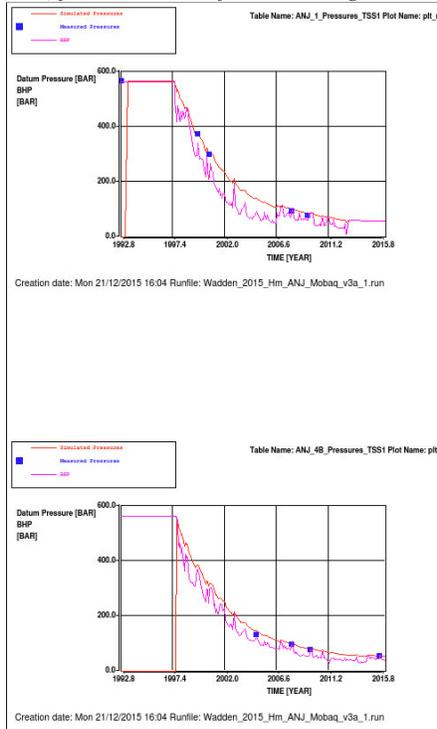
Figure 9 Simulated pressure (red line), simulated BHP (violet line) and measured down hole pressure (blue squares) for high case. Left: ANJ-1, Right: ANJ-4B.
