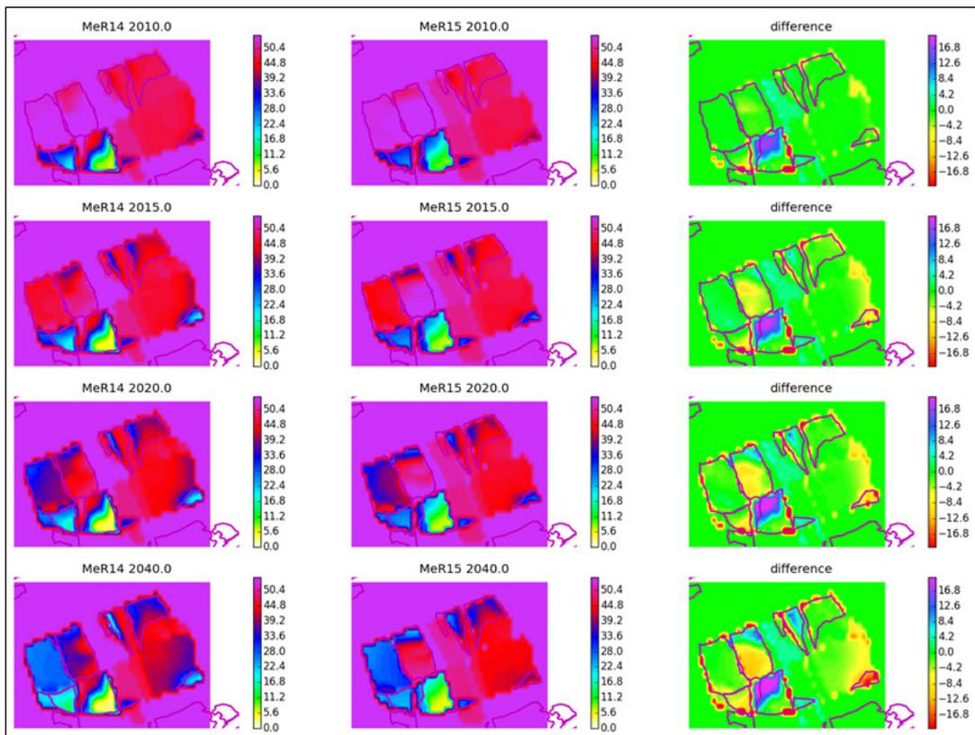
Figure 68 Modelled average reservoir pressure (MPa) of Wadden area (base case). Left column: M&R2014. Middle column: M&R2015. Right column: difference plot. Top to bottom: 2010, 2015, 2020, 2050.
