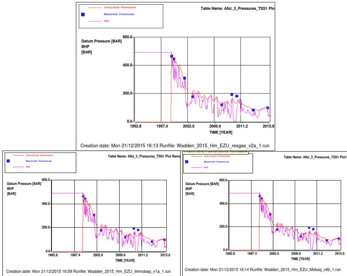
Figure 15 Simulated pressure (red line), simulated BHP (violet line) and measured (blue squares) downhole pressure data in ANJ-3. Top: base case. Left: low case. Right: high case.
