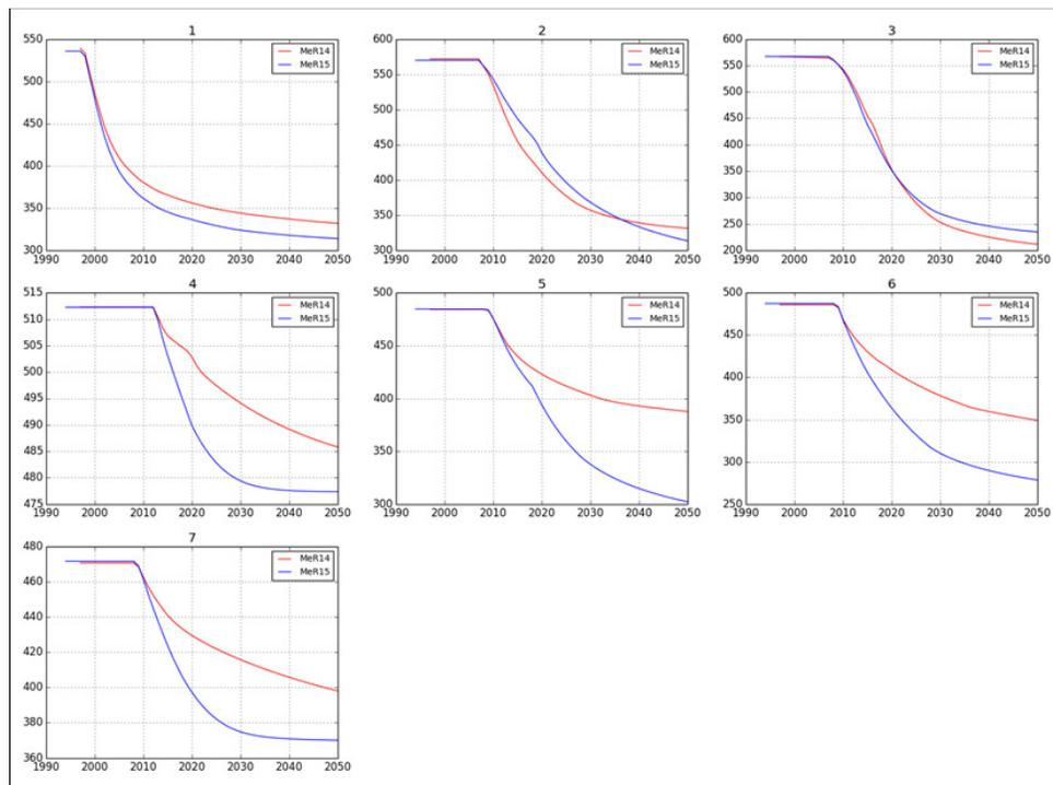
Figure 71 Average reservoir pressures per (set of) field(s), high case. Red: M&R2014, blue: M&R2015. 1 = Anjum, Ezumazijl, Metslawier, 2 = Moddergat, 3 = Nes, 4 = Lauwersoog Central, 5 = Lauwersoog East, 6 = Lauwersoog West, 7 = Vierhuizen East
