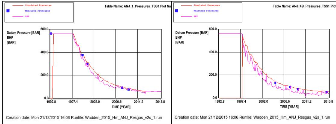
Figure 7 Simulated pressure (red line), simulated BHP (violet line) and measured down hole pressure (blue squares) for base case. Left: ANJ-1, Right: ANJ-4B.
