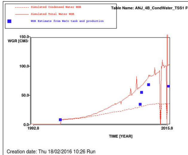
Figure 12 Simulated total WGR (red solid line), simulated condensed WGR (red dashed line) and estimated WGR from production and WaCo tank observations (blue squares) for ANJ-4B. Base case realization.
