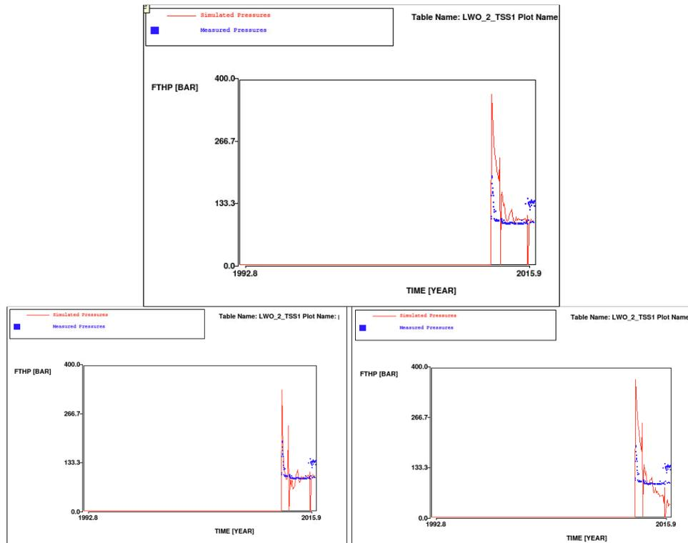
Figure 22 Simulated (red line) and measured (blue squares) flowing tubing head pressures in LWO-2. Top: base case. Left: low case. Right: high case.
