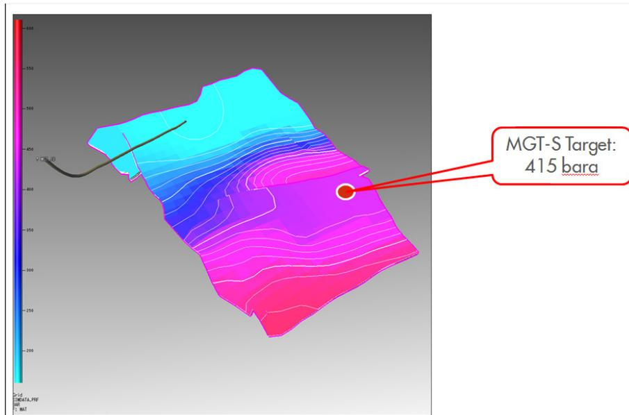
Figure 50 Base case pressure profile in the Moddergat field in 2015.
