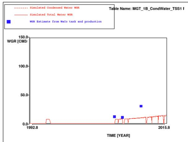
Figure 54 Simulated total WGR (red solid line), simulated condensed WGR (red dashed line) and estimated WGR from production and WaCo tank observations (blue squares) for MGT-1B. Base case realisation.
