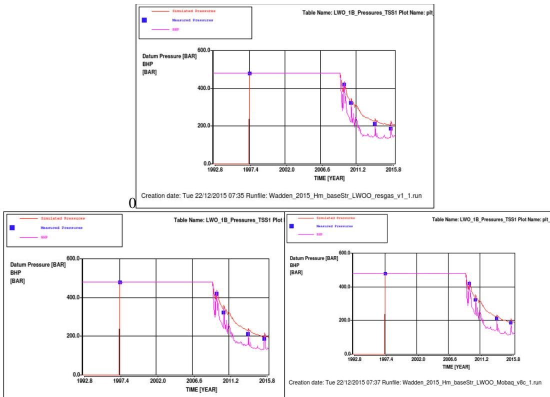
Figure 27 Simulated reservoir pressure (red line), flowing bottom hole pressure (violet line) and measured (blue squares) downhole pressure data in LWO-1B. Top: base case. Left: low case. Right: high case.
