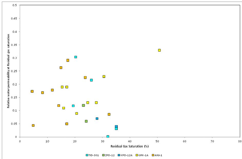
Figure 4 Relative water permeability at residual gas saturation as a function of the residual gas saturation.
