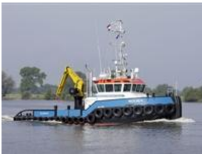
Figure 20: Example of Anchor Handling tug
