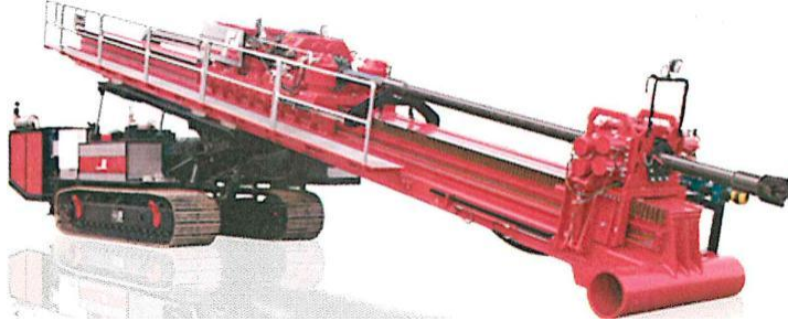
Figure 37: Typical example 250 ton drillrig
