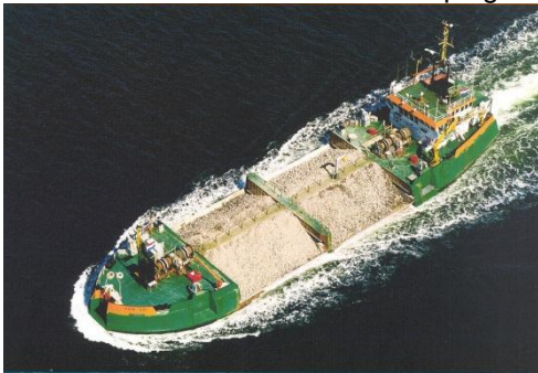
Figure 50: Typical example of a side stone dumper
