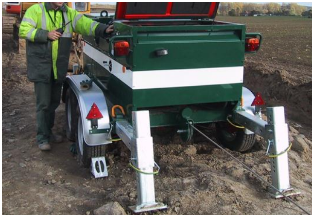
Figure 6: Typical cable hauling winch
