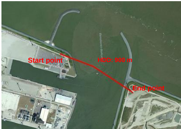
Figure 17: HDD drilling route (red line) Doekegat (Eemshaven)
