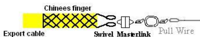
Figure 36: Chinese finger + swivel + pull wire
