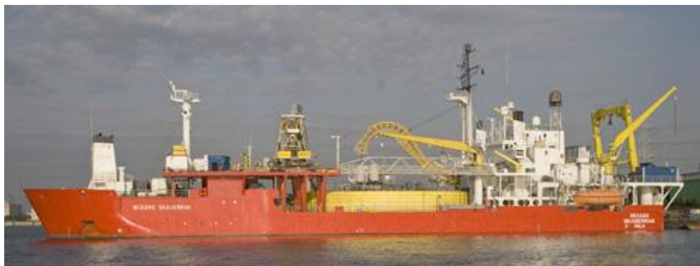
Figure 54: Typical Example Cable Lay vessel
