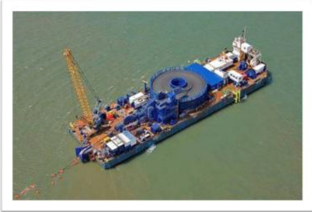
Figure 9: Cable on board an installation barge with dynamic turntable
