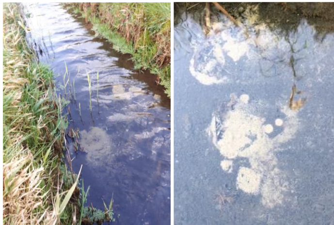
Figuur 2.6 Zandmeevoerende wellen in teensloot Standhazensedijk
