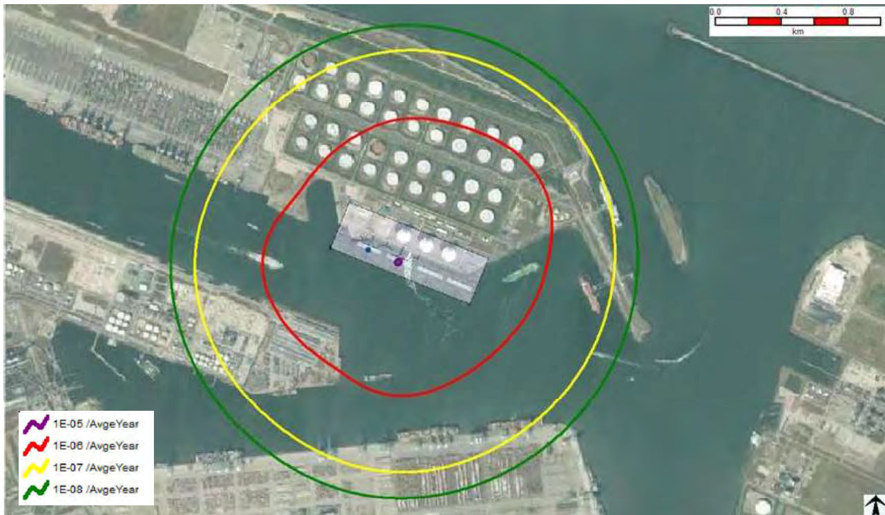
Figure 9-1: Location-specific individual risk contours for terminal phase 1 – present traffic situation
