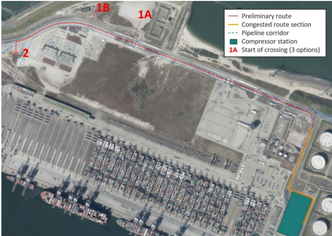
Figure 7 - Aramis onshore route overview. Various crossing locations have been analysed with 1A selected and 1B (alternate tunnel departure) and 2 (Direct Pipe) deselected.
