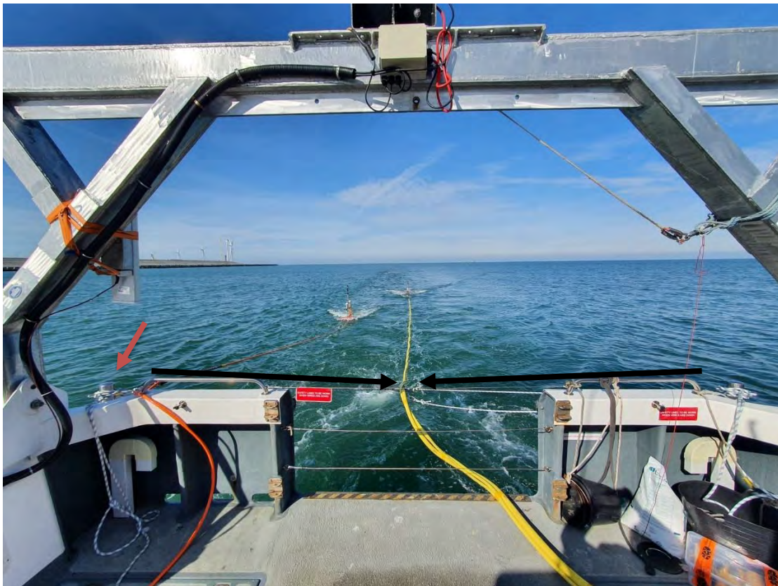
Figure 11 - Seismic spread deployed. Red arrow: streamer tow points; Black arrows: sparker tow points.
